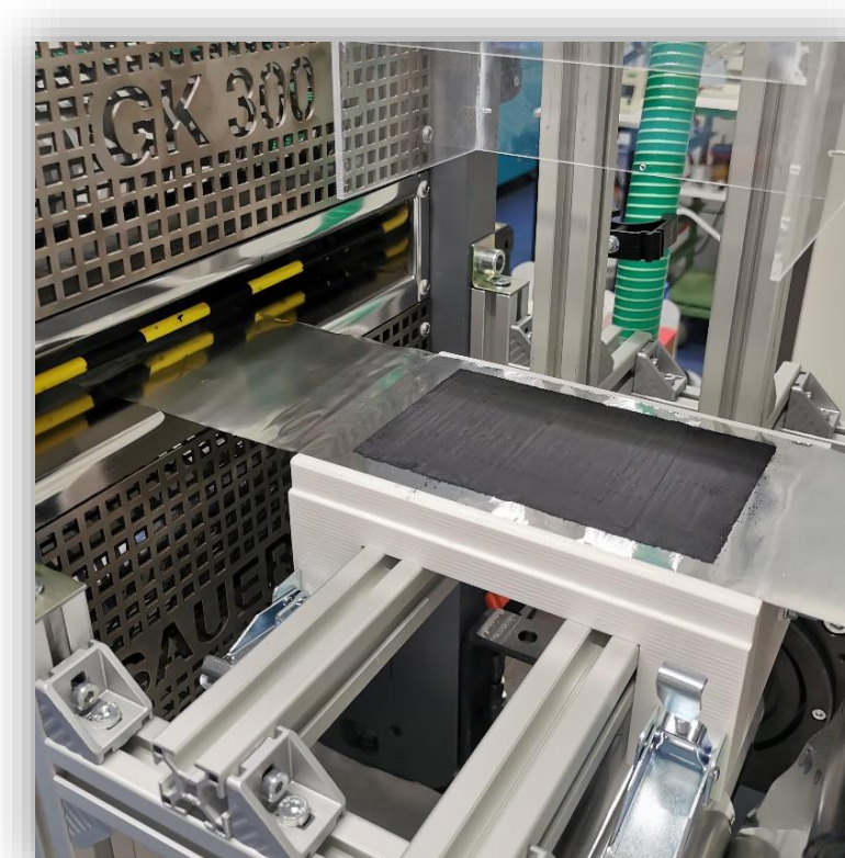
Figure 2: Solvent-free manufacturing process at AIT pilot line facilities [4]
